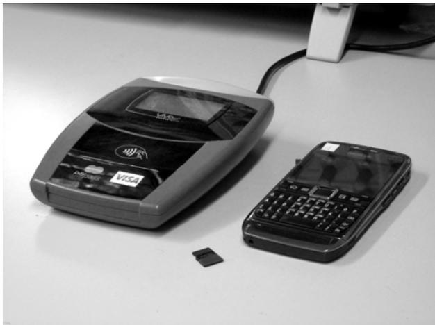
**Figure 10:** Contactless payment terminal (left) and mobile phone with micro-SD card (front)
