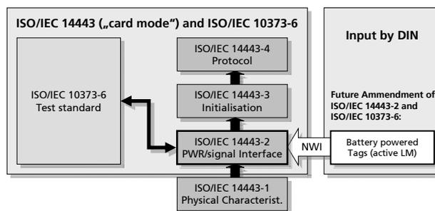
**Figure 19:** Our approach of standardising active load modulation in ISO/IEC 14443
